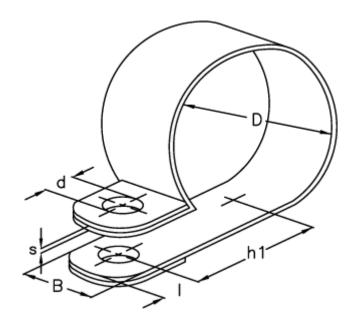
$\begin{array}{ll} d & = 10.5 \\ \text{Diameter D} = 37 \\ \text{h1} & = 33.0 \\ \text{I} & = 10.0 \\ \text{s} & = 1.0 \\ \text{Width B} & = 25 \\ \end{array}$
